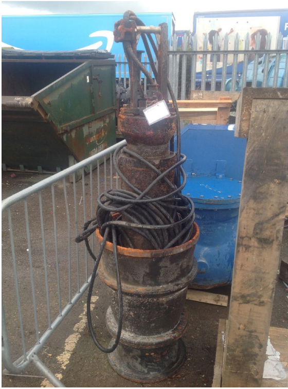
KSB AMACAN PUMP BEFORE
