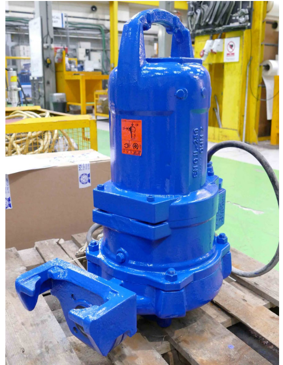
KSB KRTF PUMP AFTER
